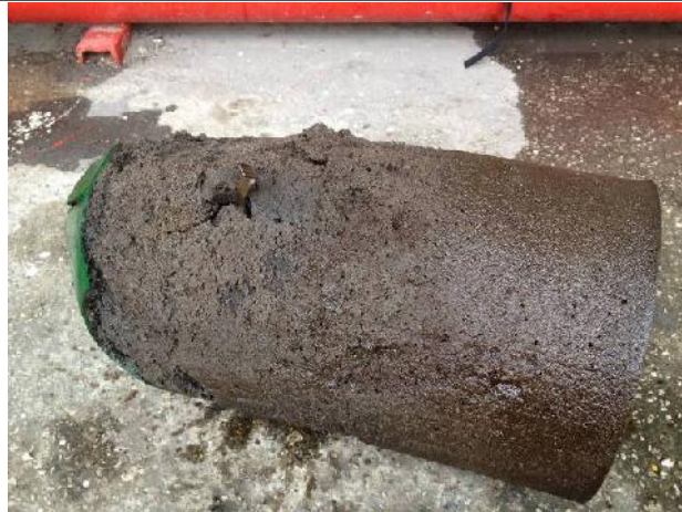
Anode Retaining Strap Embedded in Foam Body
